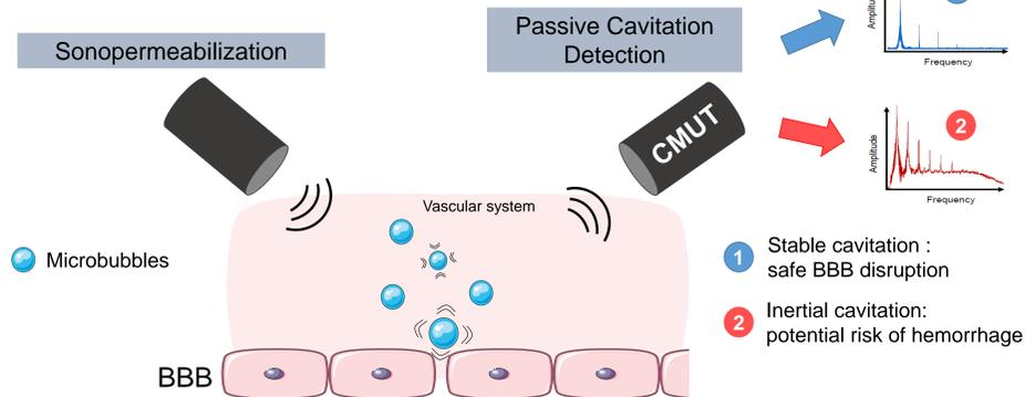
MB nonlinear response, in particular **ultraharmonics (UH)**<sup>1</sup>, can be monitored with **passive cavitation detection (PCD)** to prevent brain damages.
