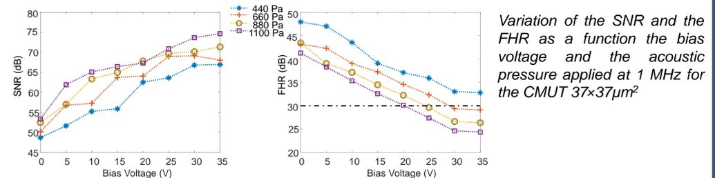
Variation of the SNR and the FHR as a function the bias voltage and the acoustic pressure applied at 1 MHz for the CMUT  $37 \times 37 \mu\text{m}^2$
