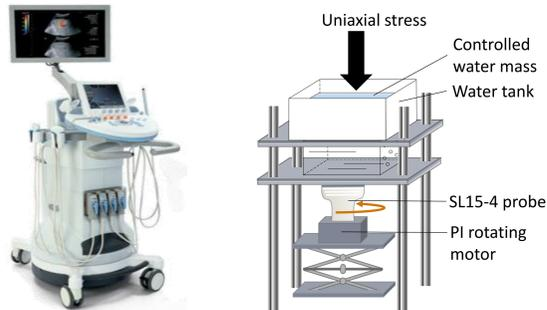
A SL15-4 probe (9 MHz central frequency, 256 elements) was rotated below the sample by using a motor, to carry out AE measurements considering SH mode waves propagating in any direction relative to the principle axis.
