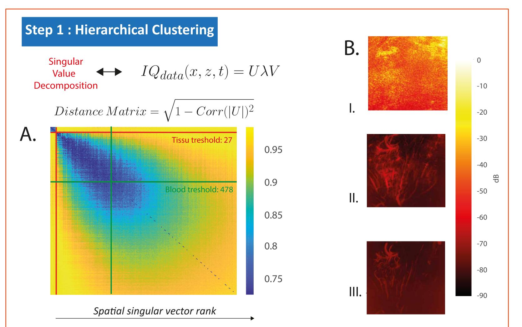
Figure 1: A. Distance matrix calculated from spatial singular vectors basis U, tresholding is obtained with hierarchical clustering; B. Power Doppler of the three subspace resulting from clustering: I. Tissue, II. Blood, III.Noisy blood.
