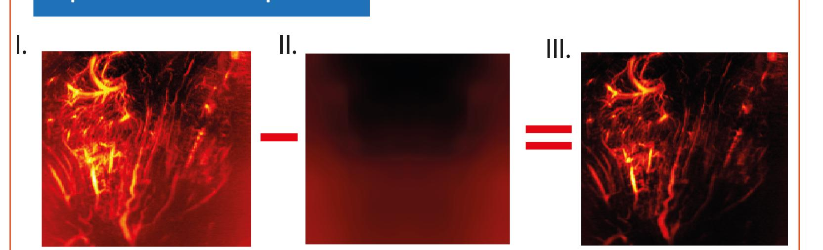
Figure 2: Noise biass suppression: I. Power Doppler of blood + noisy blood , II. Noise profil obtained from half lower energetic spatial singular vectors with median filtering and fft2, III. Denoised blood obtained by substraction (I) - (II).
