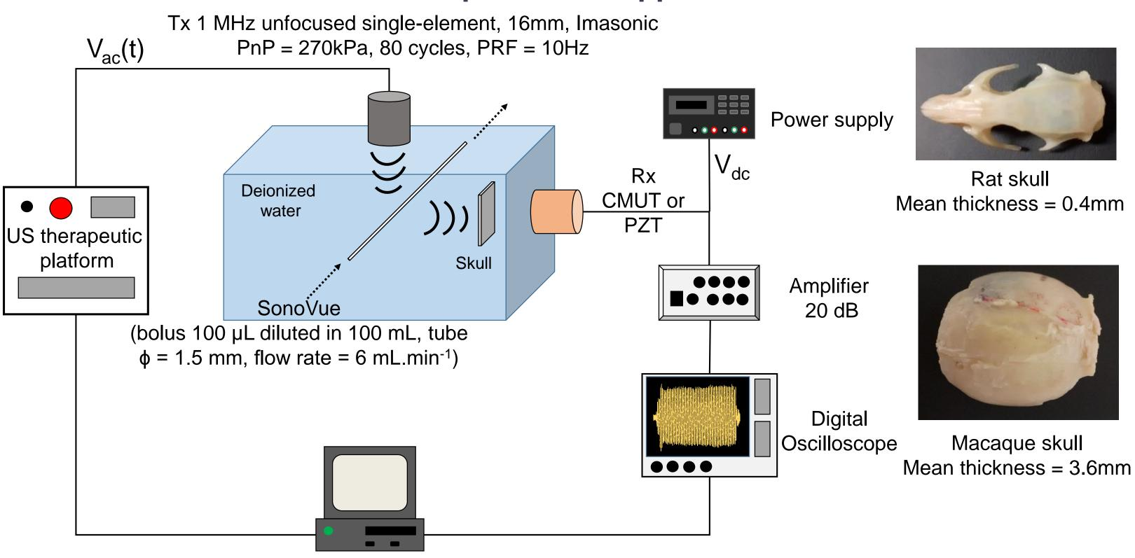
The frequency response from circulating MB was evaluated by calculating area under curve ratio (AUCR) between the signal from MB and the signal backscattered by the water-filled tube for harmonic  $((n+1)f_0, n=2 \text{ to } 6) \text{ and } UH (0.5nf_0, n=2 \text{ to } 5).$
