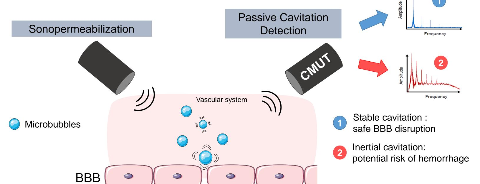
MB nonlinear response, in particular ultraharmonics (UH)<sup>1</sup>, can be monitor with passive cavitation detection (PCD) to prevent brain damages.
