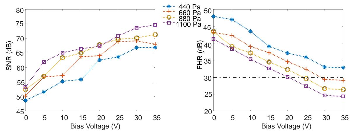
Variation of the SNR and the FHR as a function the bias voltage and the acoustic pressure applied at 1 MHz for the CMUT 37×37µm<sup>2</sup>
